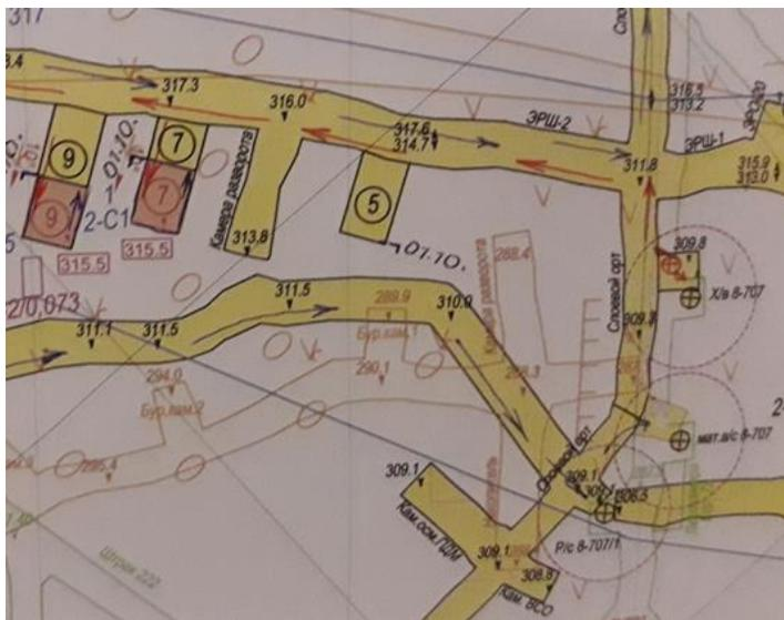
**Figure 4.** Layout of mine workings at the site for capability demonstration test of the tracked XLPD low-profile LHD
