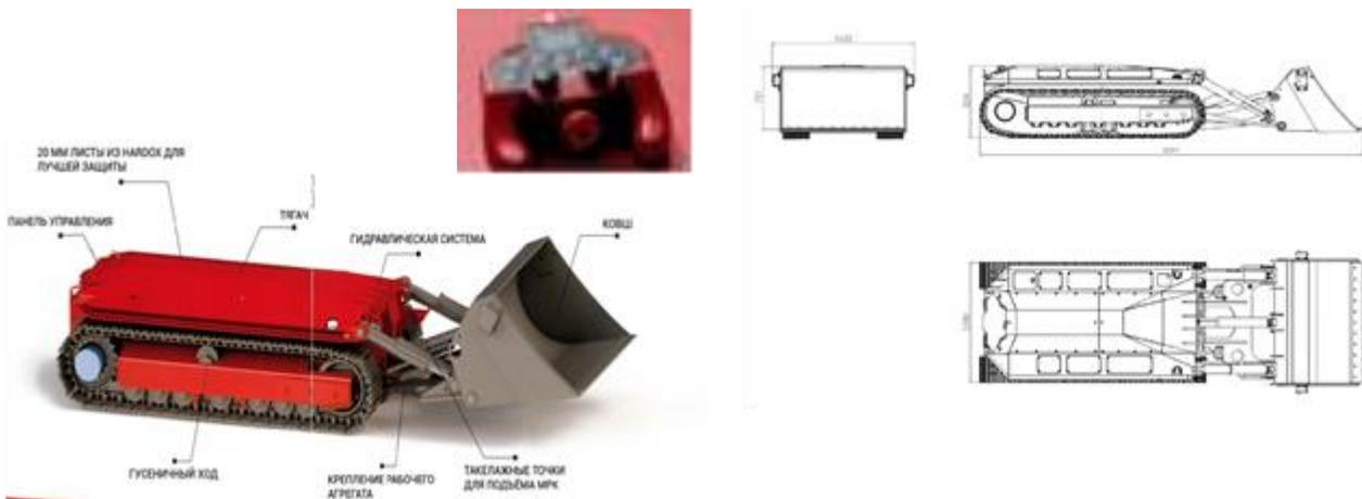
**Figure 3. Exterior view of the XLPD low-profile robotic LHD:**
