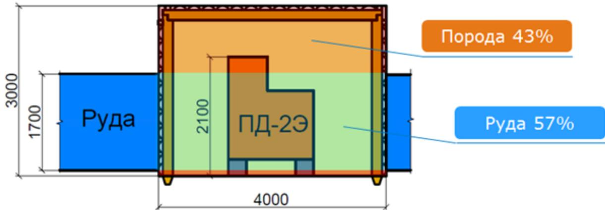
**Figure 2.** Typical cross-section of the stopes when the PD-2E unit is used for ore haulage
