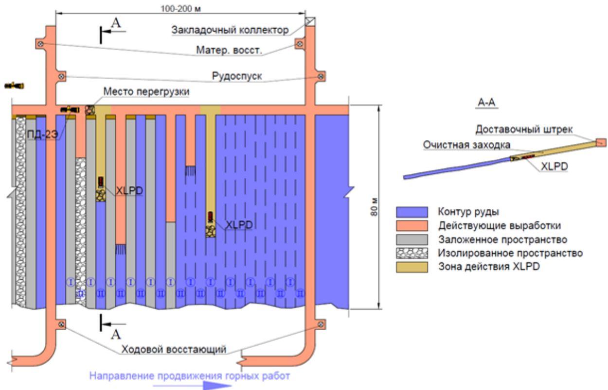
**Figure 7.** Recommended block development and extraction plan using the XLPD LHD
