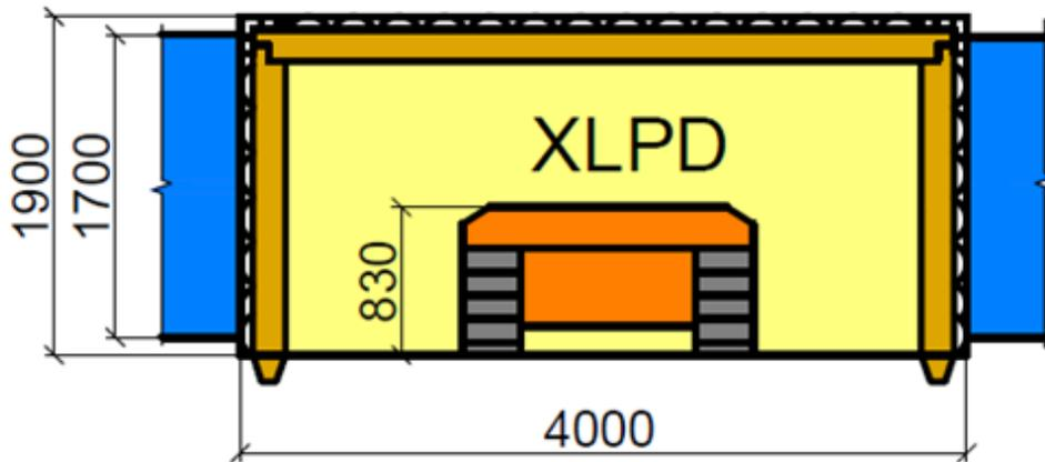
**Figure 6.** Mine working cross-section with the post-and-bar support with the tracked XLPD low-profile LHD used for ore haulage
