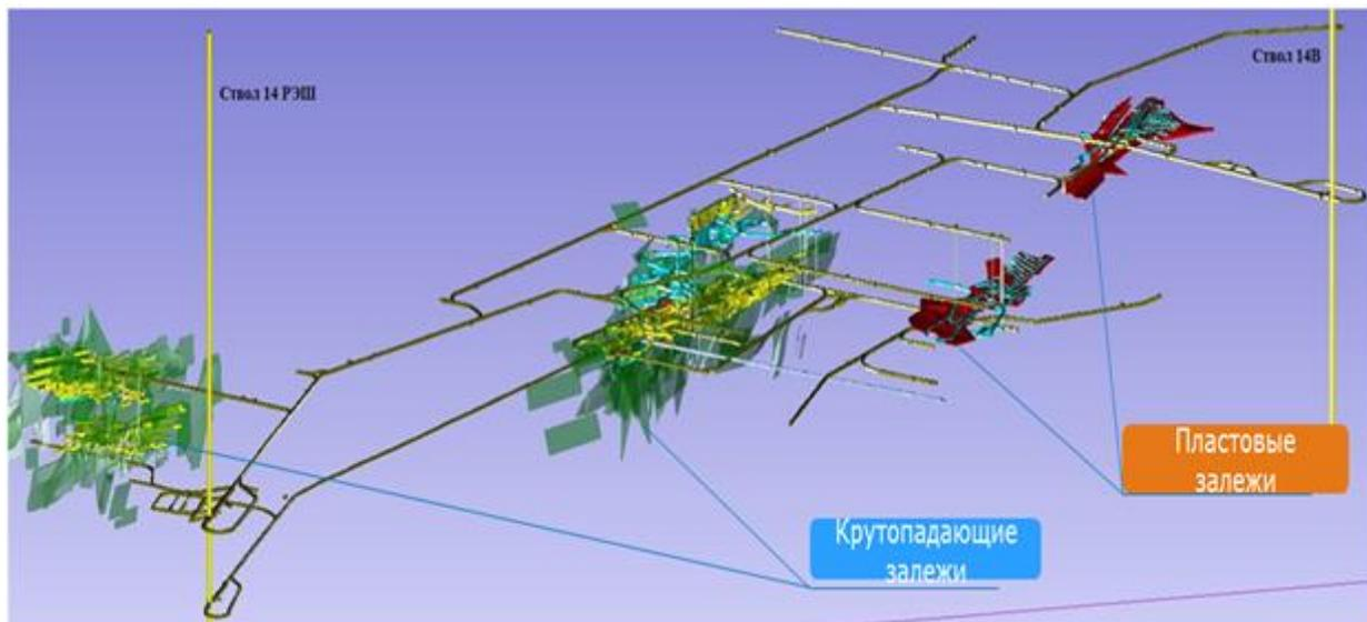
**Figure 1.** 3D model of mine workings and ore bodies at Levels 6 and 7 in Mine No.8 with indication of the steeply dipping and bedded ore bodies
